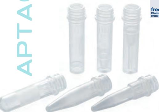
Graduated, in transparent polypropylene, tubes only. Resistance to temperatures from -85 °C to +121 °C, autoclavable. Suitable for centrifuge use to RCF 25.000 g. DNase, RNase and pyrogen free.
