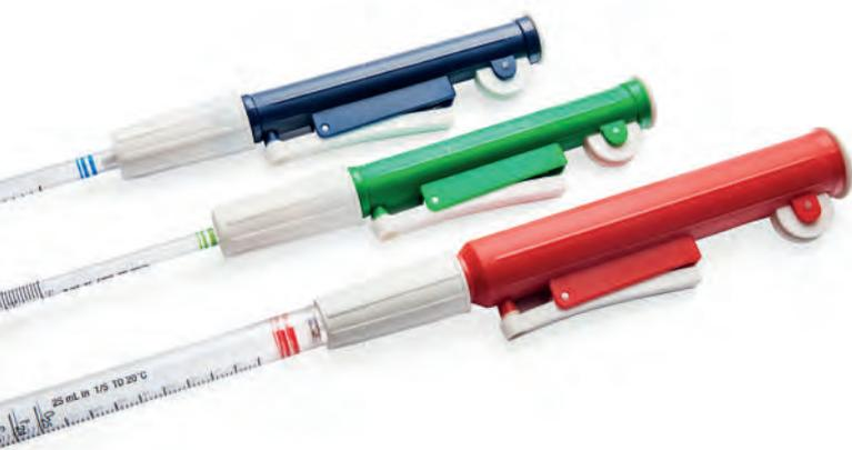
In polypropylene, for any kind of pipettes, both glass and plastic. Suction and dispensing are achieved by rotating the wheel. Complete and rapid discharge of liquid by pressing the lever.
