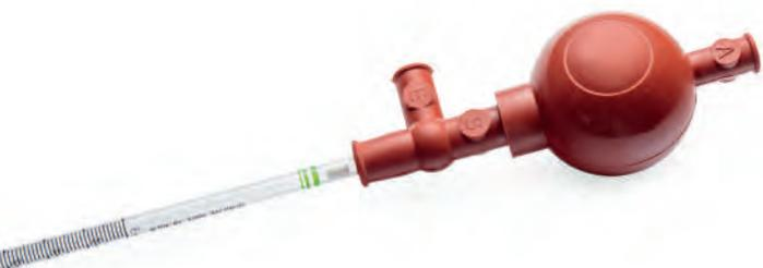
Pipettes filler in red rubber provided with three spheric glass valves: air exhaust, liquid filling and dispensing. Universal model, it can be used with all pipettes, both plastic and glass.
