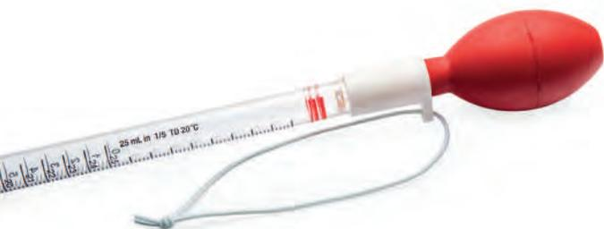
In red rubber and silicone, it prevents from mouth pipetting and, therefore, from any contamination risk. Suitable for pipettes up to 25 ml.
