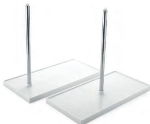
Extendable stand with rectangular polypropylene bases and chrome-plated steel rods. The rods, 250 mm in length and 12 mm in diameter, are modular and can be screwed together to achieve greater lengths. The stands can be used with funnel holders art. 10801 and 10802. Supplied with two rods.
